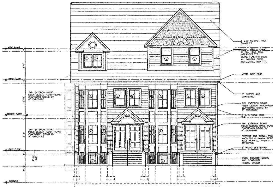
FRONT ELEVATION BUILDING D
