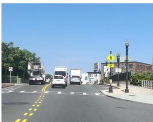
**Installed curb extension and Rapid Flash Beacon** at Saratoga and Barnes Street, adjacent to Orient Height MBTA Station in East Boston.
