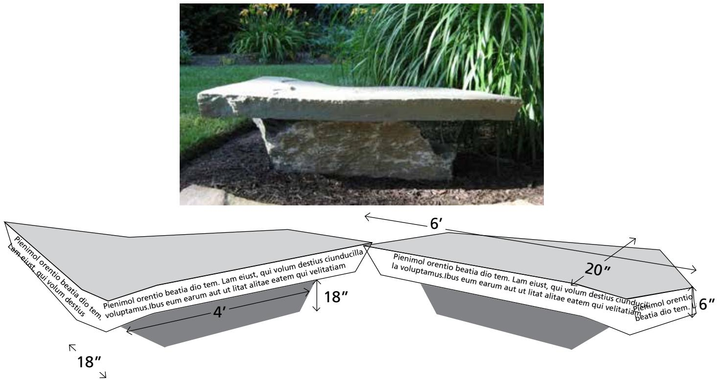
All rough except the white areas which would be sawn. .75"H letters will be sandblasted and filled with black or white lithichrome paint. Template for tops required.
