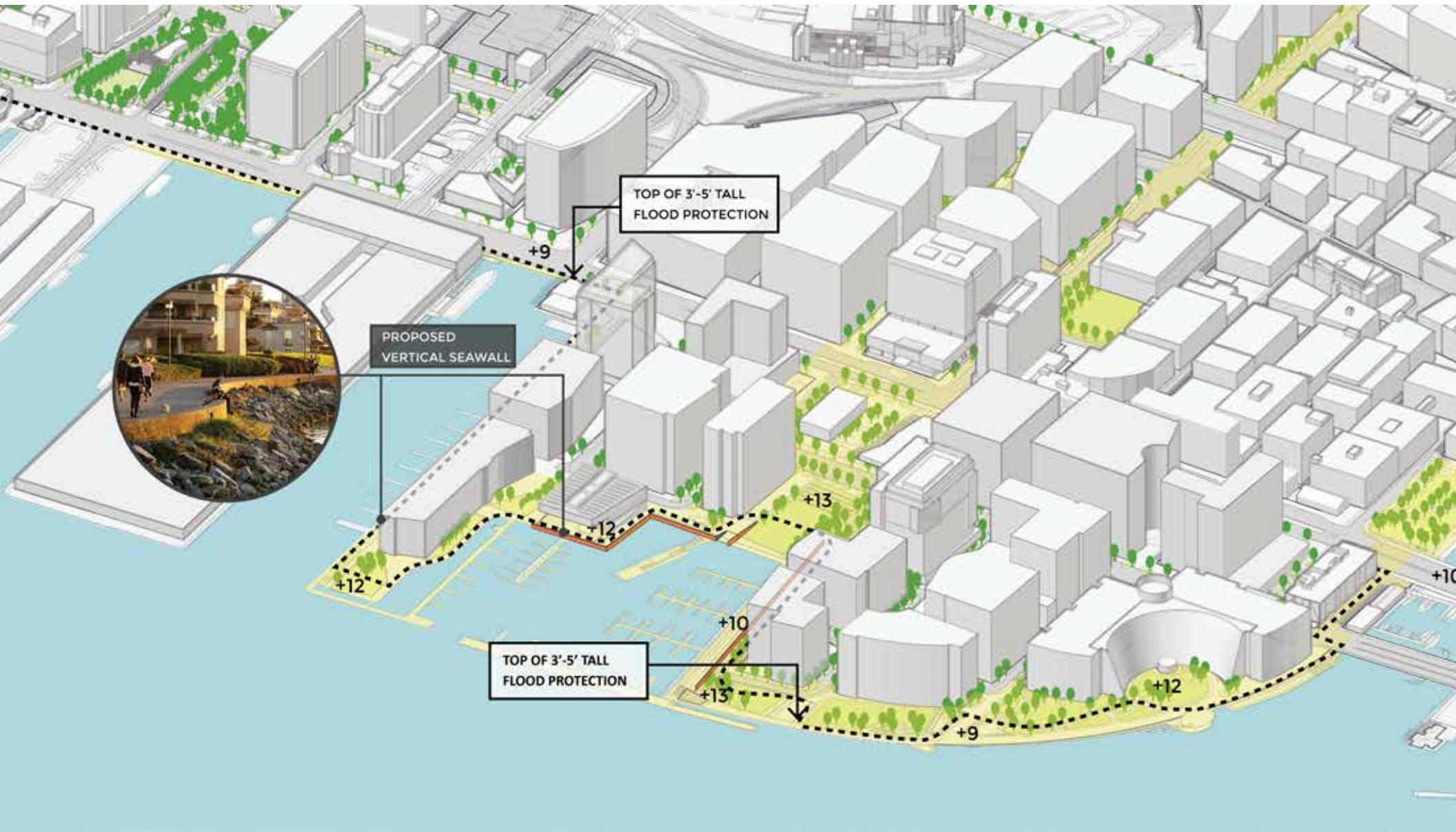
Design concept prototypes for flood protection alignment Option A along the shoreline of the Waterfront. Option A makes use of existing space to reduce flood risk.
