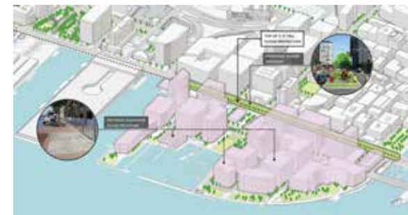
Design concept prototypes for flood protection along Seaport Boulevard and dry floodproofing of seaward structures
