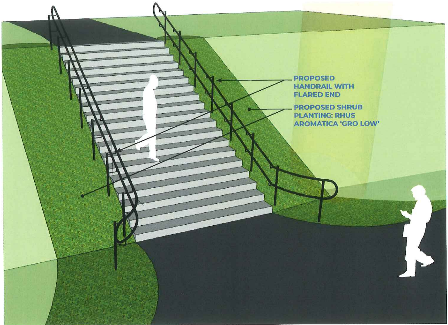
View of rehabilitated pond stairs with shrub plantings and handrails
