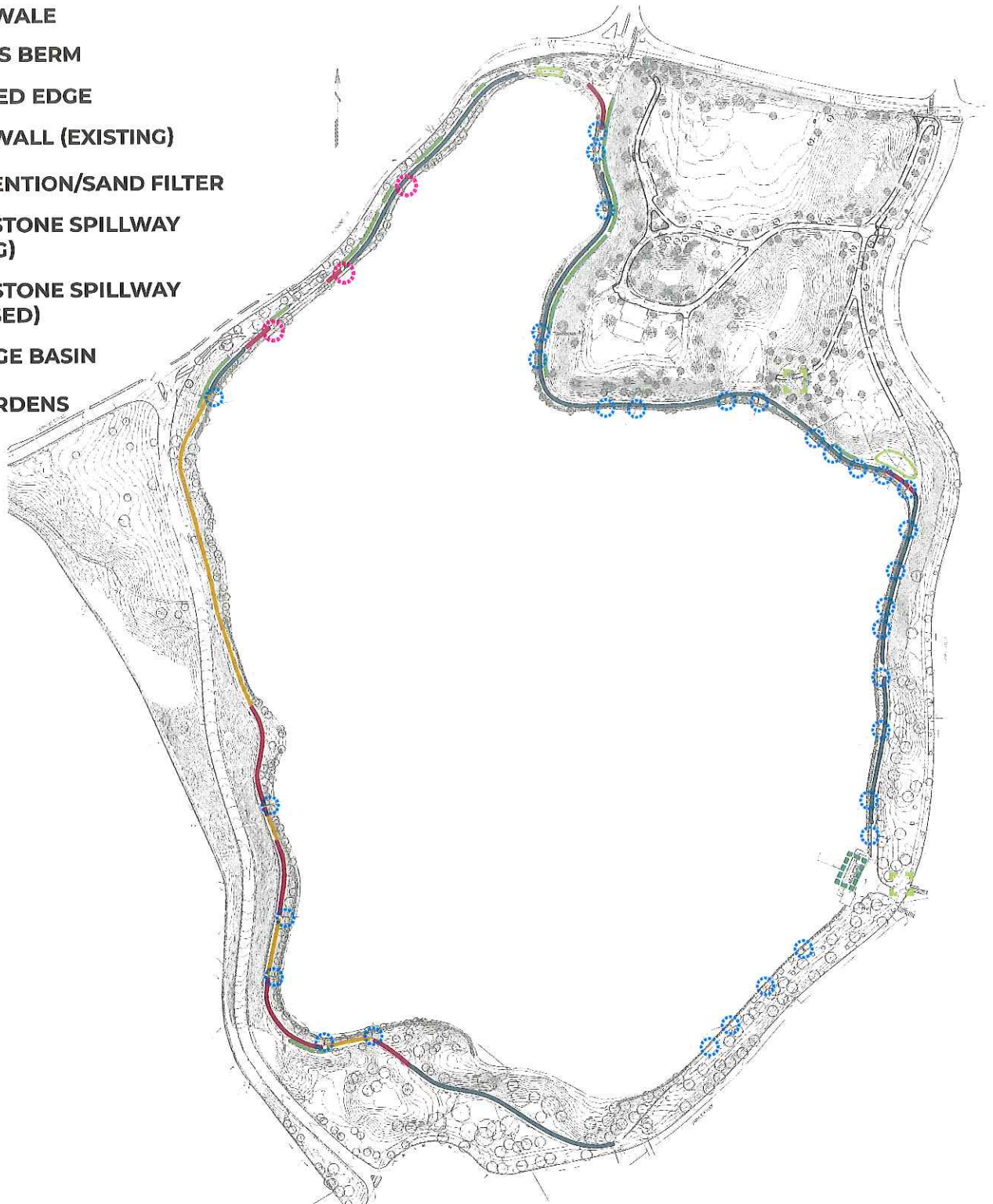
Proposed stormwater management interventions
