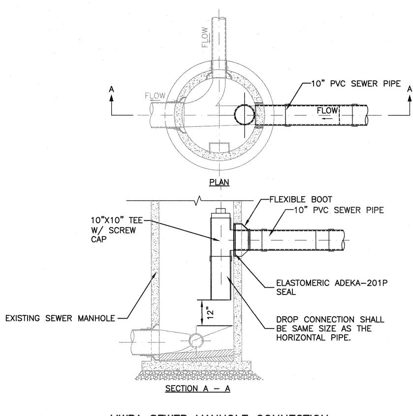
MWRA SEWER MANHOLE CONNECTION DROP MANHOLE CONNECTION NOT TO SCALE
