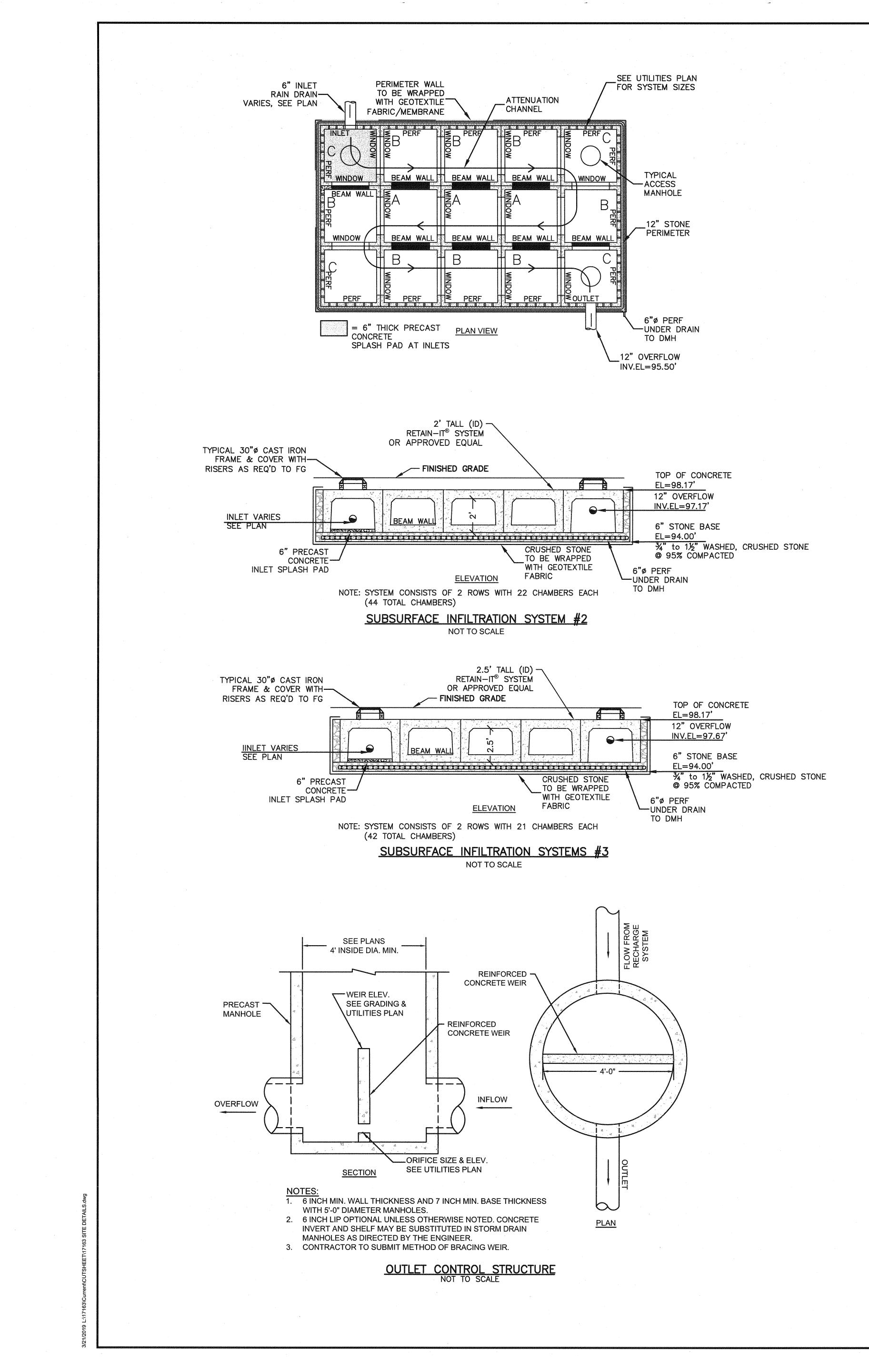
MIN. COVER TO RIGID PAVEMENT, H SPRINGLINE -----4" FOR 12"-24" PIPE 6" FOR 30"-60" PIPE
