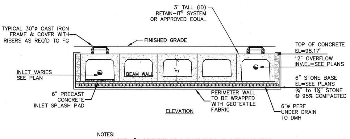
1. SYSTEM #4 CONSISTS OF 3 ROWS WITH 12 CHAMBERS EACH (36 TOTAL CHAMBERS)
