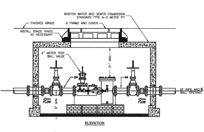
WATER METER PIT DETAIL NOT TO SCALE
