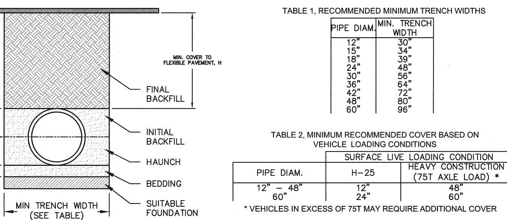
1. ALL PIPE SYSTEMS SHALL BE INSTALLED IN ACCORDANCE WITH ASTM D2321, "STANDARD PRACTICE FOR UNDERGROUND INSTALLATION OF THERMOPLASTIC PIPE FOR SEWERS AND OTHER GRAVITY FLOW APPLICATIONS", LATEST ADDITION, WITH THE EXCEPTION THAT THE INITIAL BACKFILL MAY EXTEND TO THE CROWN OF THE PIPE. SOIL CLASSIFICATIONS ARE PER THE LATEST VERSION OF ASTM D2321. CLASS IVB MATERIALS (MH, CH) AS DEFINED IN PREVIOUS VERSIONS OF ASTM D2321 ARE NOT APPROPRIATE BACKFILL MATERIALS.
