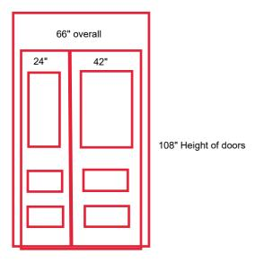
Replace double doors with one larger 42" door and 24" sidedoor to meet ADA code for the lift replacement. Detail and design to match
