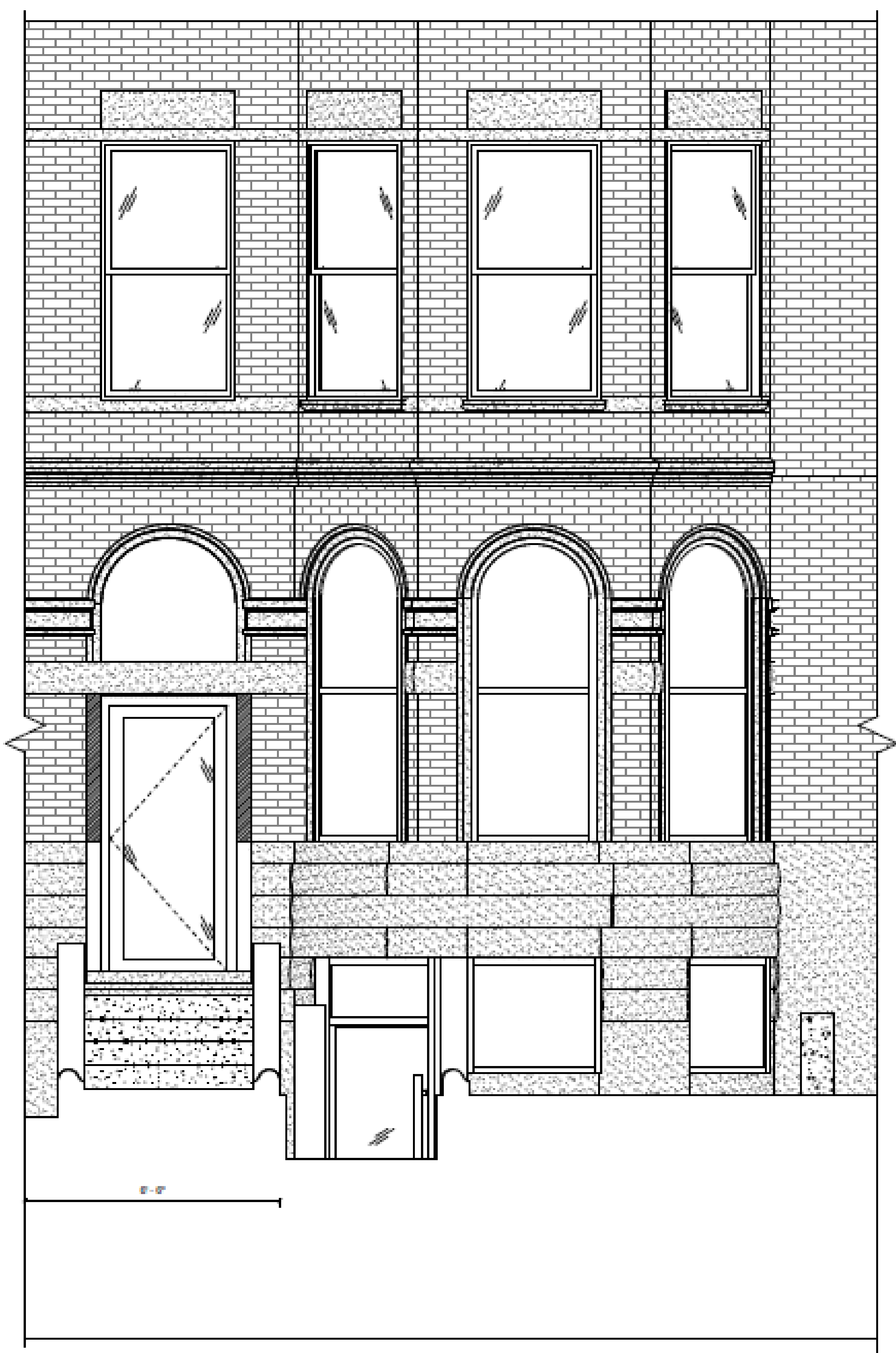
3 SECTION - EXISTING FRONT FACADE NORTH 1/2" = 1'-0"
