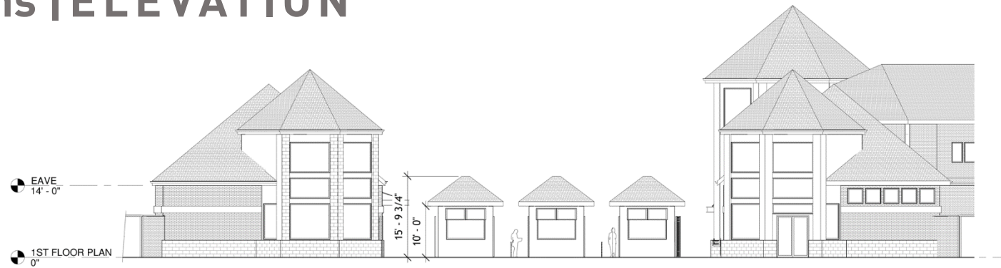
ticket booths with individual 9:12 sloping roof "hats"
