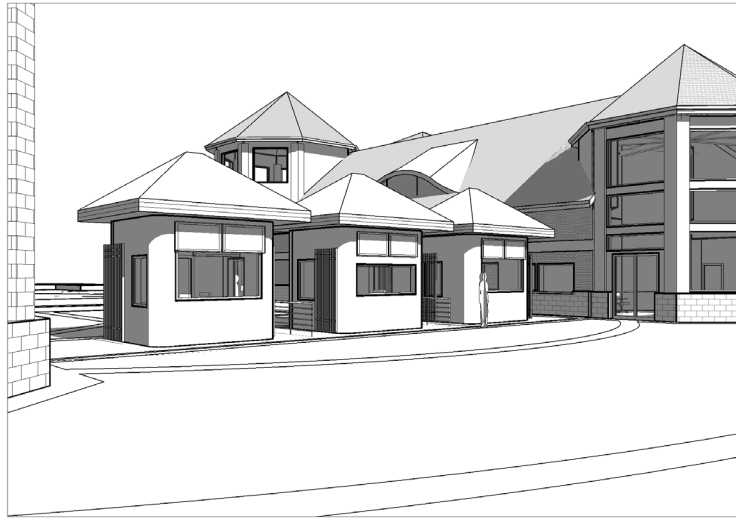
ticket booths with individual 9:12 sloping roof "hats"
