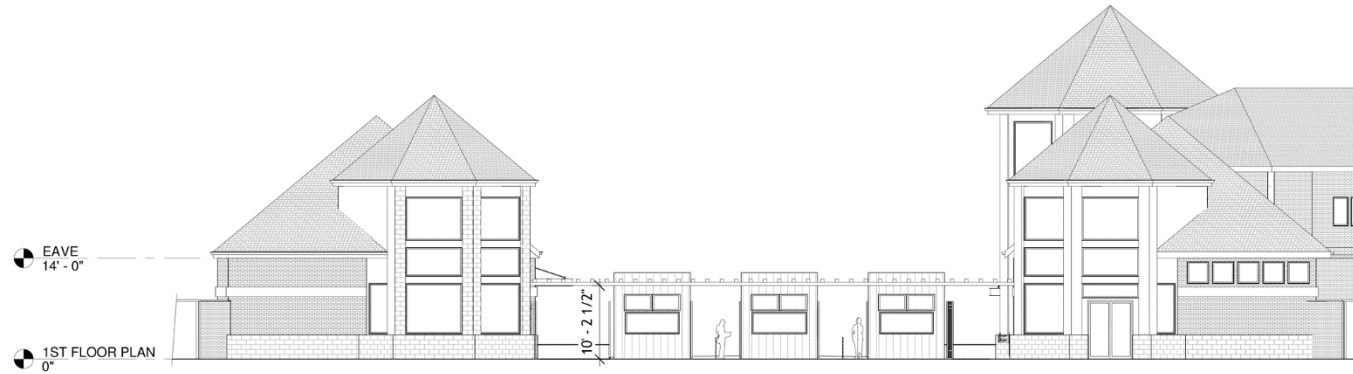
ticket booths with connecting flat roof arbor
