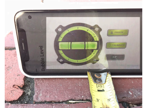
PITCH AWAY FROM BUILDING = 3.4° = 5.94% slope
