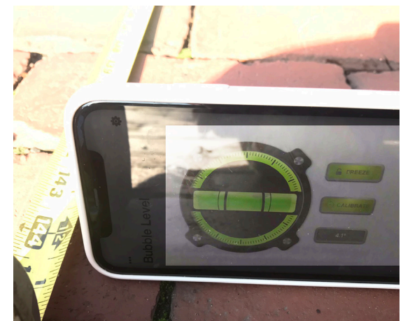
PITCH AWAY FROM BUILDING = 4.1° = 7.17% slope
