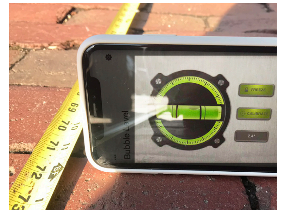
PITCH AWAY FROM BUILDING = 2.4° = 4.19% slope
