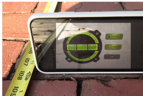
PITCH AWAY FROM BUILDING = 2.6° = 4.54% slope
