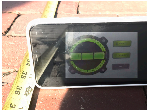
PITCH AWAY FROM BUILDING = 3.6° = 6.29% slope
