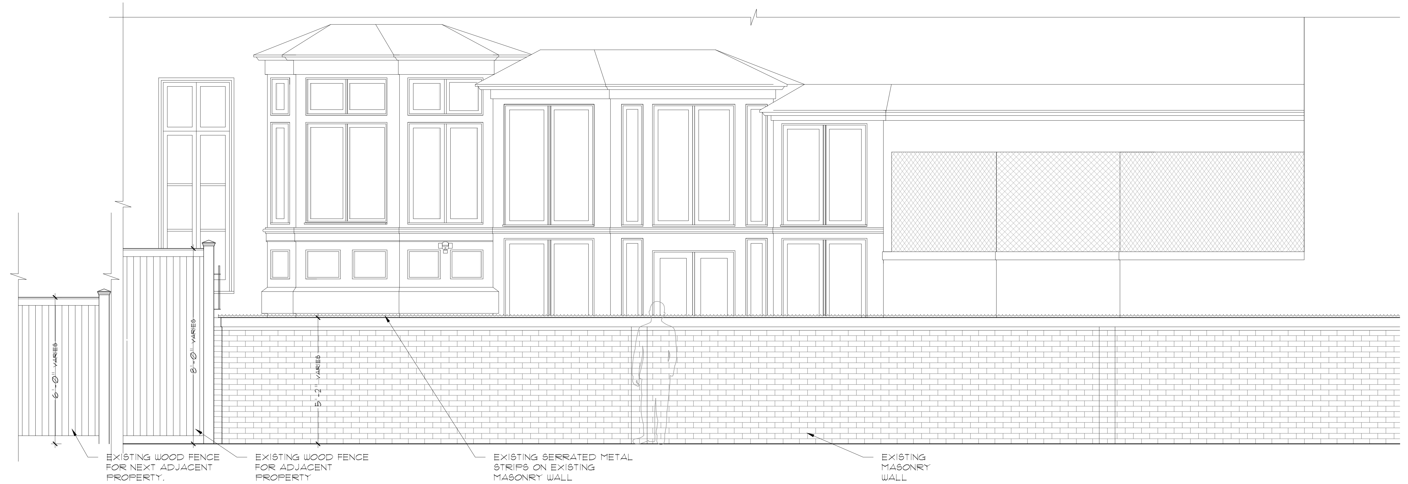
1 EXISTING GARDEN WALL ELEVATION - EXTERIOR FULL: 1/2" = 1'-0", HALF: 1/4" = 1'-0"
