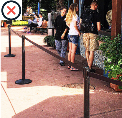
This is not allowed! It lacks cane-detectable leading edge.
