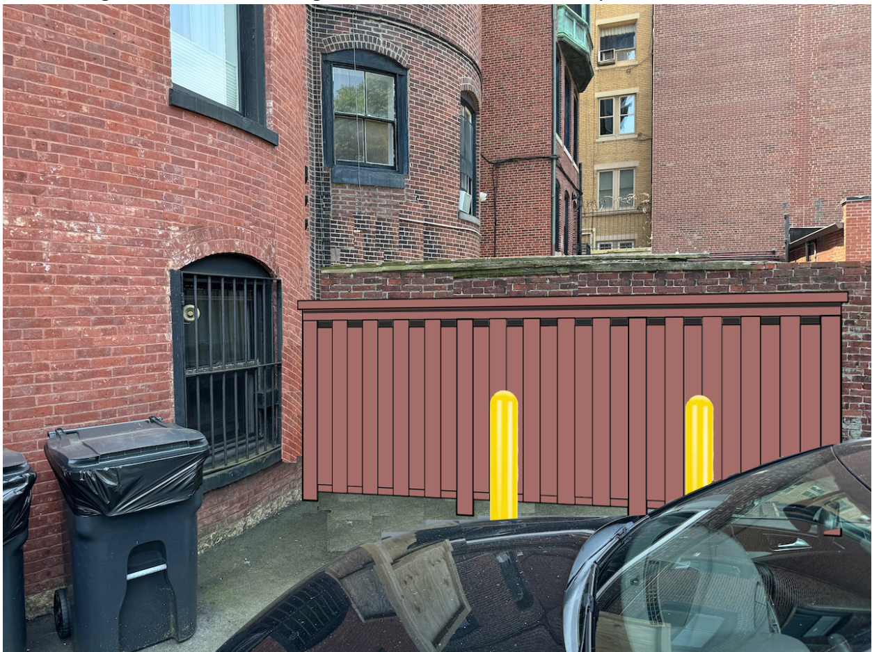
Three new Heat Pumps will be screened with a 6'-8" high, board-on board wooden fence
