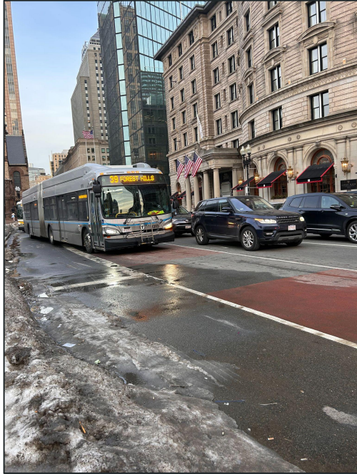
Bus lane allows for bus to exit stop without impacting general vehicle movement
