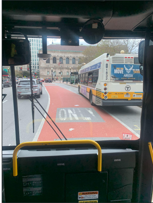
Bus lane prevents bus movement from conflicting with vehicle movement
