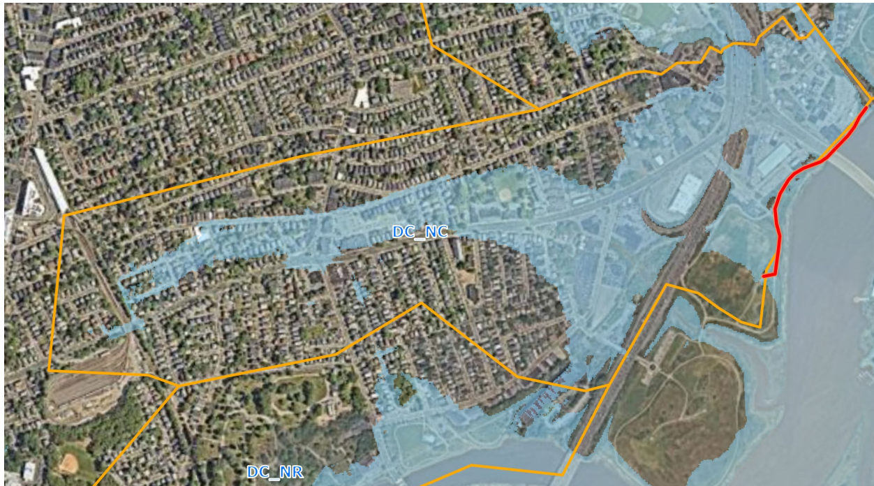
Figure 61. Alternative DOR6 is a levee and in-water floodwall system through Pope John Paul II Park and along the Neponset Trail on the Neponset River which manages coastal flood risk within the DC_NC model area.
