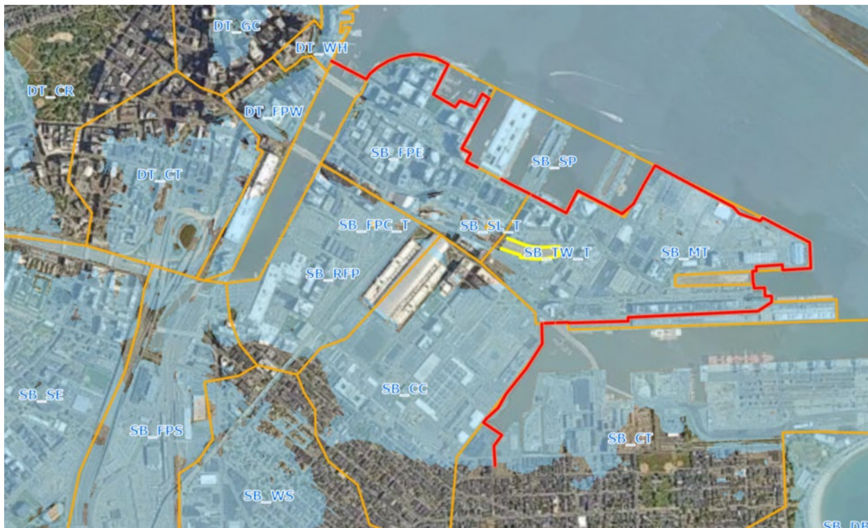
Figure 50. Alternative SB3 (in red) provides a complete flood risk management solution to elevation 14' NAVD88 for all model areas south and west of the alignment.
