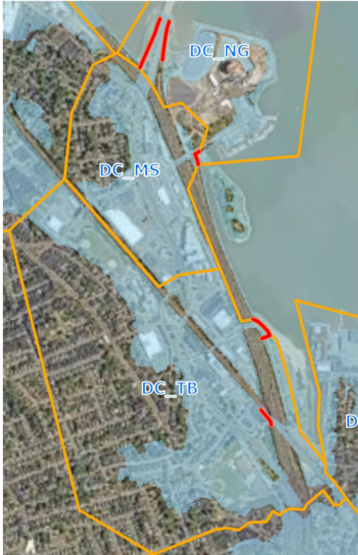
Figure 60. Alternative DOR4 builds upon DOR3, with the addition of a pair of floodwalls alongside Morrissey Boulevard between its underpass at I-93 and the Beades Bridge and a small berm at Victory Road and the I-93 North offramp to Freeport St/Dorchester.
