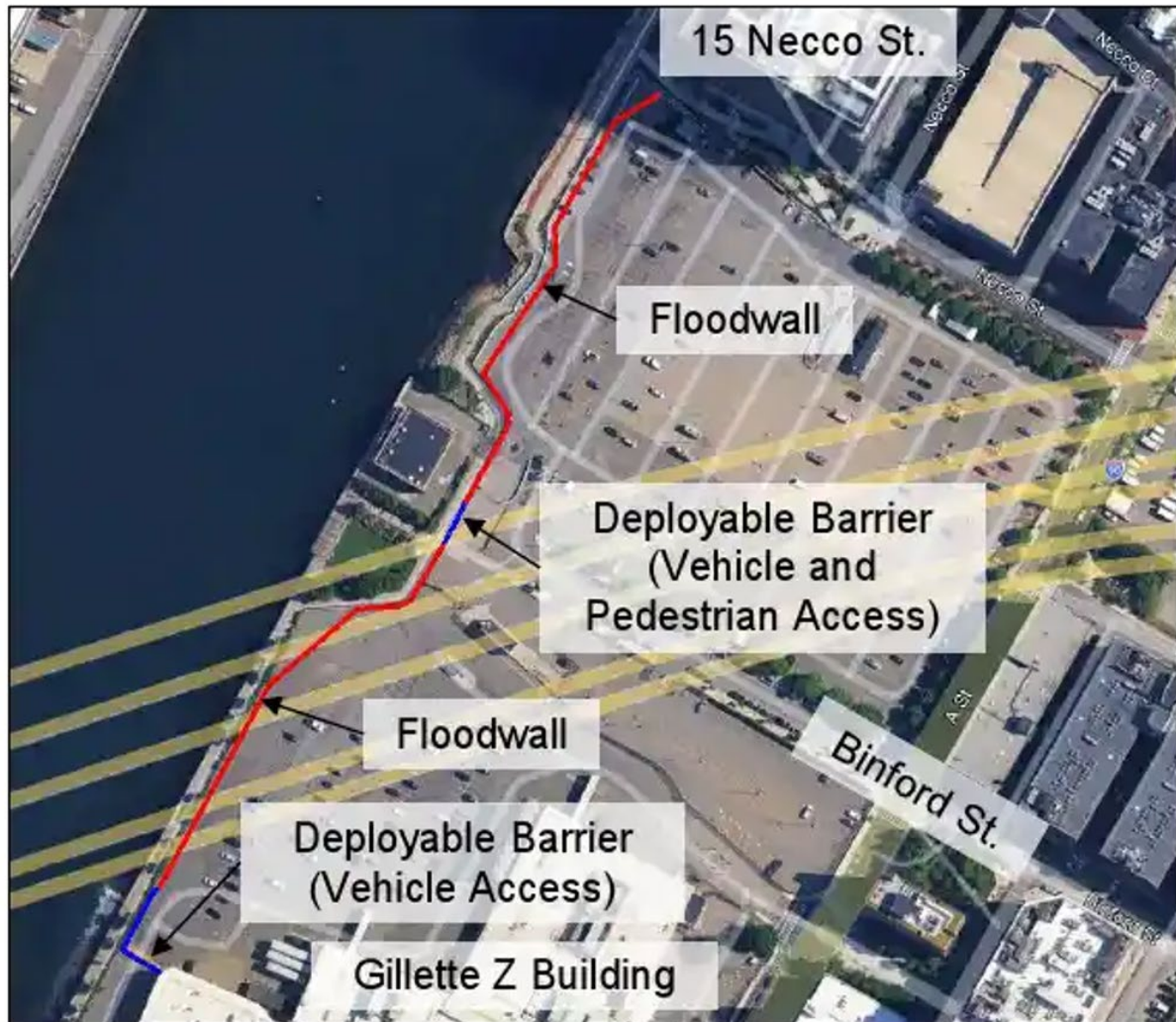
Figure 55. 15 Necco Street to the Gillette Z building floodwall and deployable barrier system.
