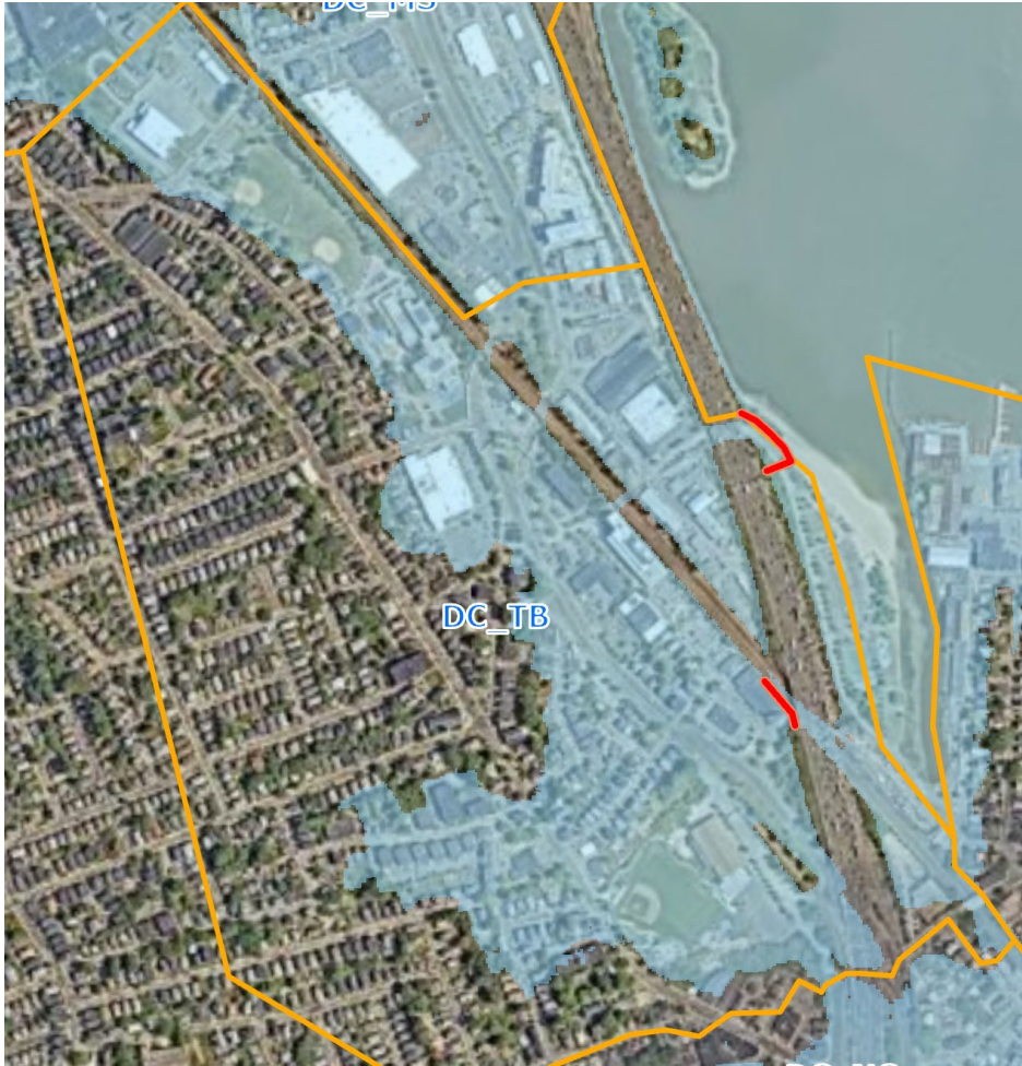
Figure 59. Alternative DOR3 provides flood risk management within model area DC_TB with a levee at the north end of Tenean Beach that prevents coastal flooding through the flood entry pathway at the Conley Street underpass and a floodwall along the south side of the rail corridor that ties into high ground at its north end and the I-93 embankment at its south end.
