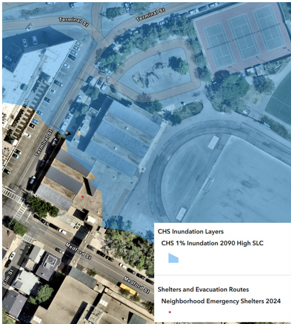
Figure 37. The Charlestown Community Center, considered for dry floodproofing, and the 2090 best estimate 1-percent AEP floodplain under the USACE High SLC scenario.
