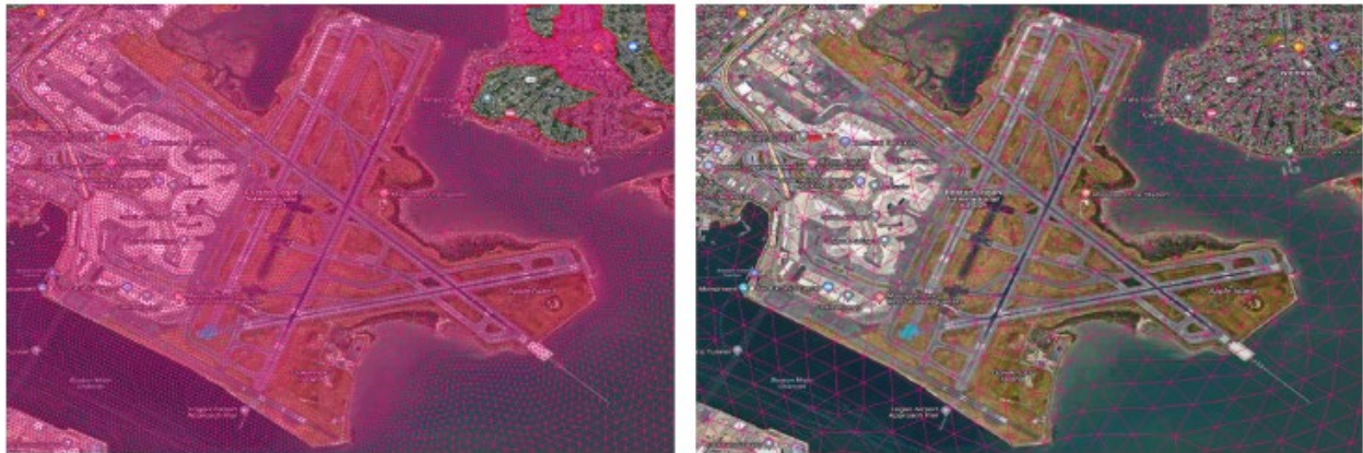
Figure 23. Comparison element resolution near Logan Airport between the MC-FRM (left) and NACCS (right) ADCIRC meshes.
