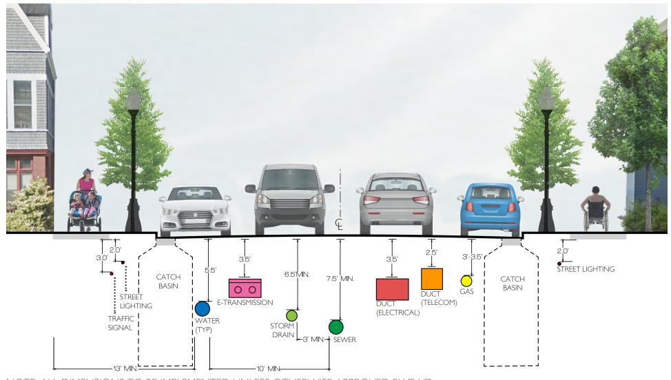
NOTE: ALL DIMENSIONS TO BE IMPLEMENTED UNLESS OTHERWISE APPROVED BY PWD. UTILITIES MAY NEED TO OFFSET AROUND MANHOLES & CATCH BASINS. IF NEEDED, E- TRANSMISSION CAN GO UNDERNEATH ELECTRICAL DUCT.
